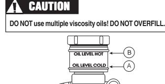
Figure 45. Transmission Reservoir
